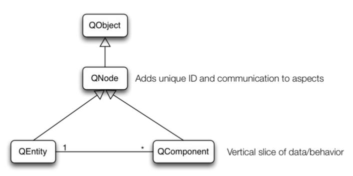
Simulated object. Aggregates components
